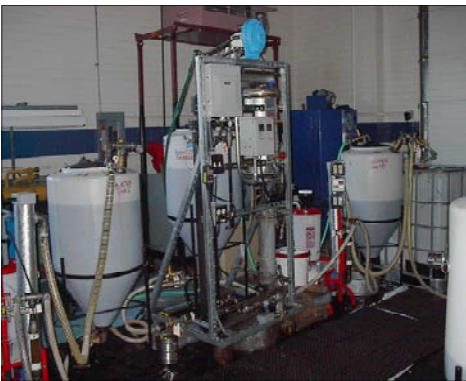
Small biodiesel generation unit with methanol stripper and wash tanks
